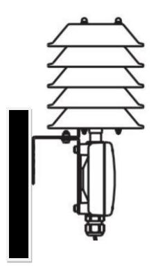
The sensor should be mounted in the same way shown, the plate gaps opening should be towards down side.
